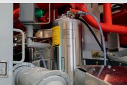
Spray tank with compressed air connection for easy cleaning of the hopper by moistening with release agent beforehand
