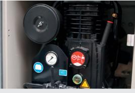
The compressor provides compressed air for various applications, e.g. cleaning
