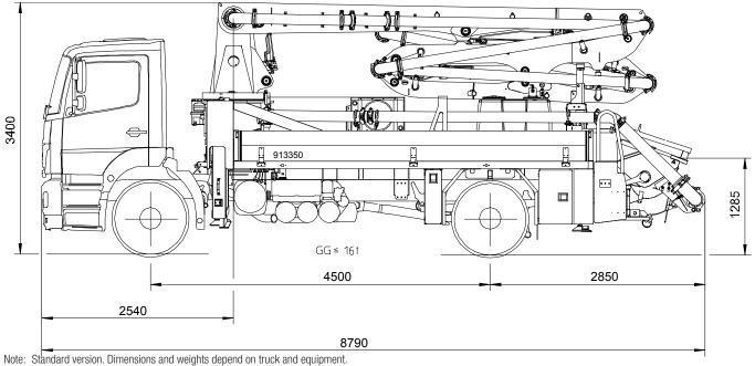
Note: Standard version. Dimensions and weights depend on truck and equipmen Dimensions in mm, MB-Axor 1828 as example. For illustration only.
