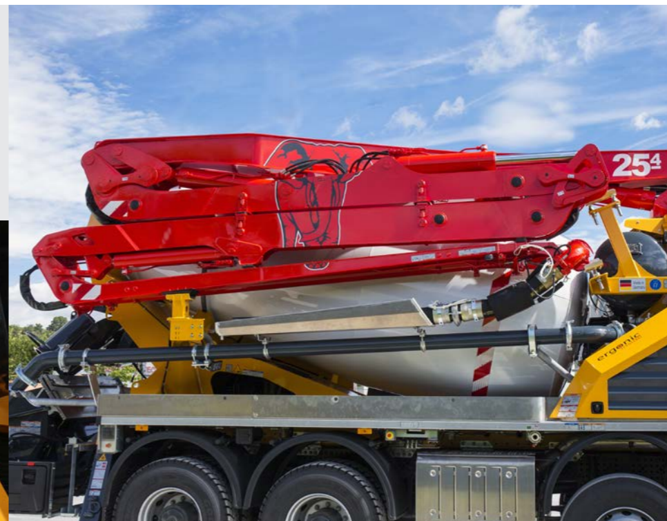
The 4-arm placing boom offers optimised slip characteristics and maximum reach
